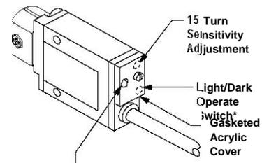
"AID" Indicator LED Lights when the sensor sees its own modulated light and pulses at a rate proportional to the strength of the received light signal.
